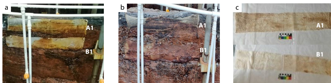
Fig. 10 The photos of Ami-gauze after different attaching time of (a) 4 days and (b) 48 days on the Nanhai I shipwreck hull; (c) The samples after desorption.
